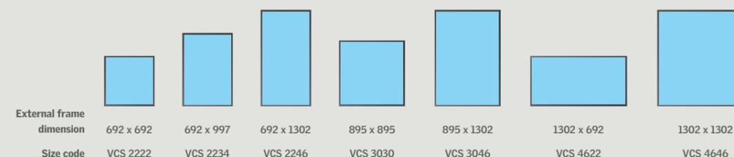
All sizes in mm. Width x Height. Manual and solar powered skylights can only be installed as per orientation depicted above. Custom-made flashing required. Raising the installation pitch to 10° may be preferred for the best aesthetic appearance. Below this pitch you are likely to experience water ponding on the glass.
