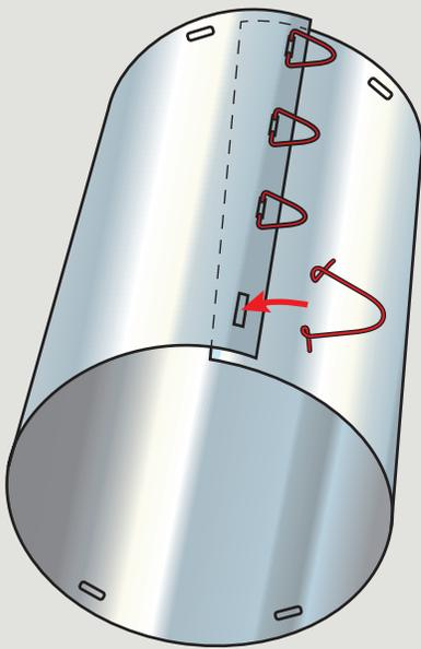
**ENGLISH:** Assemble the rigid tunnel sections with tunnel clips provided.
