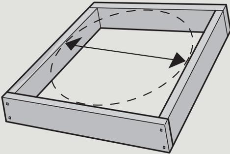
**ENGLISH:** To make the flashing fit properly on the curb, the curb and roofing material dimensions must be less than the flashing clearance, ie  $20\frac{7}{8}'' \times 20\frac{7}{8}''$  (530 mm x 530 mm).
