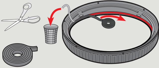
**ENGLISH:** Attach pile gasket to the pivot ring as shown.
