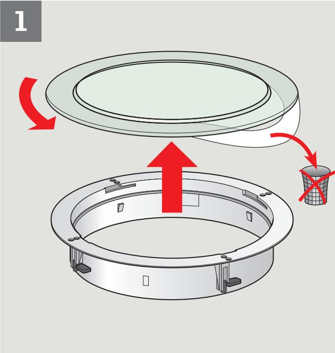
**ENGLISH:** Carefully remove the primary diffuser from the ceiling ring. Rotate the diffuser to disengage.
