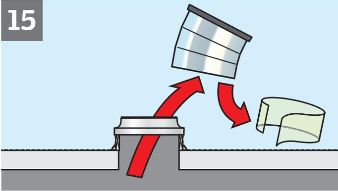
**ENGLISH:** Remove the elbow and remove protective film from upper elbow.
