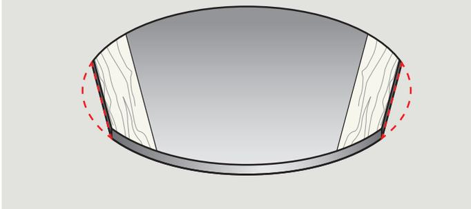
**ENGLISH:** From the inside, locate the nail indicating the center of the sun tunnel in the ceiling, mark circle and cut rough opening in the ceiling as shown.
