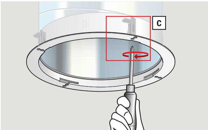
**ENGLISH:** Tip the plastic pins down into hidden position **A**. Insert the ceiling ring assembly. Avoid distortion of the ceiling ring causing the diffuser not to fit smoothly **B**.
