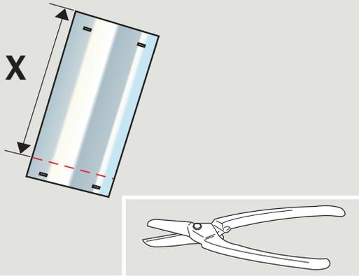
**ENGLISH:** With one rigid tunnel section, cut the section to length.
