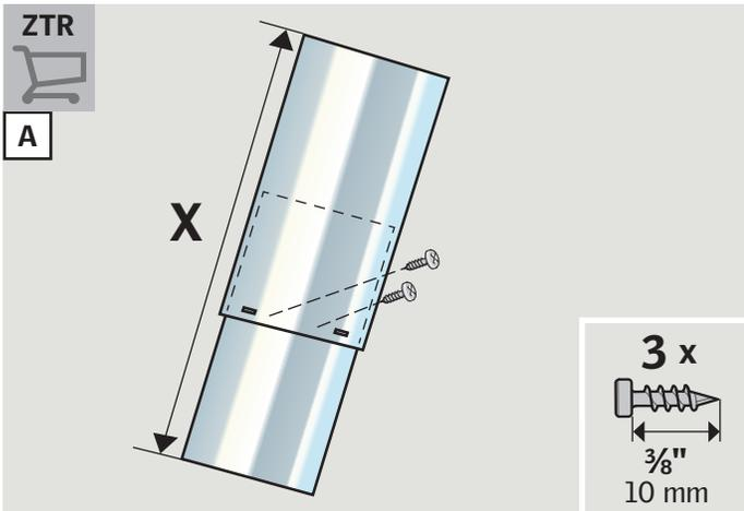
**ENGLISH:** With two tunnel sections, reduce the length of the tunnel assembly by increasing overlap. Secure the joint with three of the 3/8" (10 mm) screws **A**.
