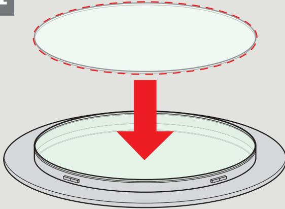
**ENGLISH:** Install the secondary diffuser disc onto the primary diffuser.
