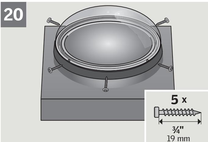
**ENGLISH:** Align holes; install and secure the dome with the 3/4" (19 mm) screws provided. Do not overtighten the screws.
