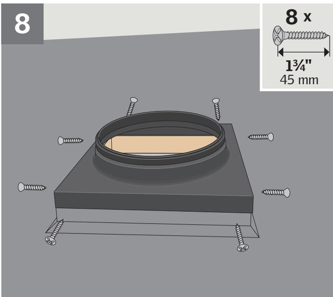
**ENGLISH:** Install and secure the flashing with  $1\frac{3}{4}''$  (45 mm) screws provided.
