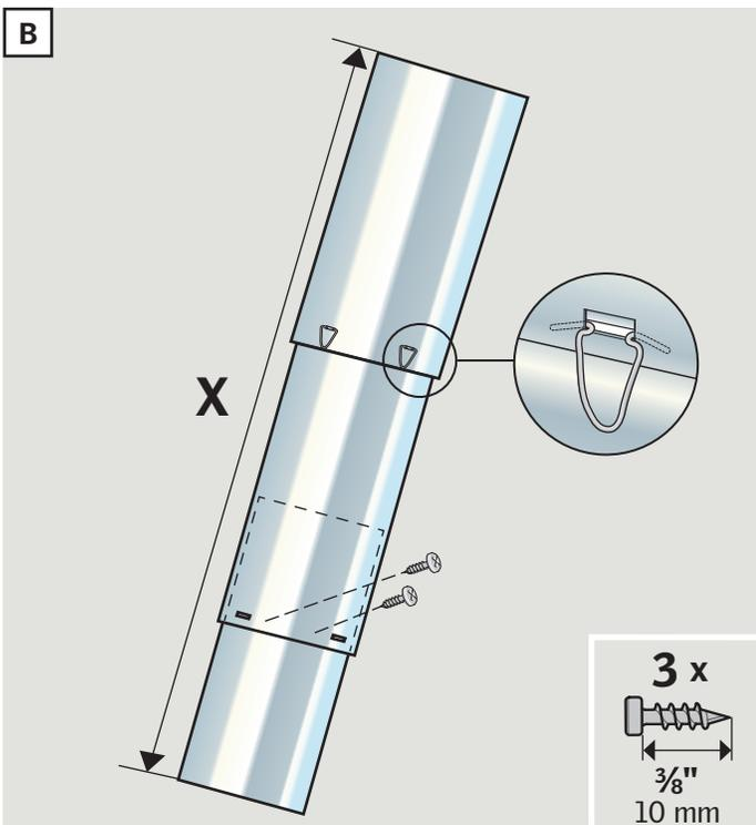
**ENGLISH:** With more tunnel sections, assemble the upper sections with the tunnel clips provided and reduce the length of the tunnel assembly by increasing overlap at the bottom. Secure the joint with three of the 3/8" (10 mm) screws **B**.
