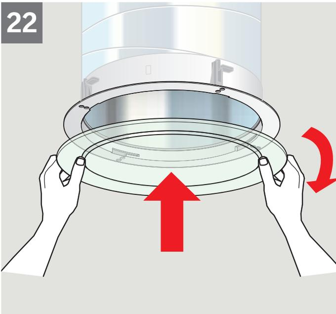
**ENGLISH:** Install the diffuser assembly by aligning the notches and rotate to secure.
