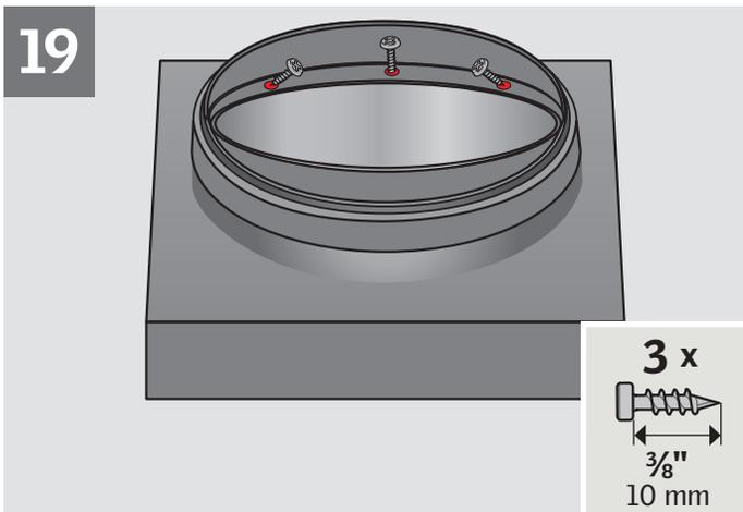
**ENGLISH:** Seat the pivot ring with the tunnel assembly into the flashing. Secure with screws if needed.
