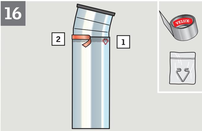
**ENGLISH:** Connect the rigid tunnel section with the upper elbow, fitting the rigid tunnel section to go on the outside of the upper elbow. Secure and tape joints with tunnel clips and tape provided **1**, **2**.
